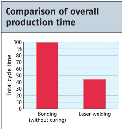
**Fig. 2. Cleaning, curing and sealing the exhaust gas outlet are eliminated in plastic laser welding**
