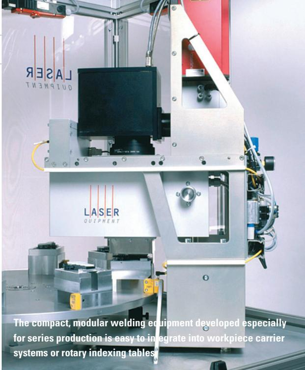
The compact, modular welding equipment developed especially for series production is easy to integrate into workpiece carrier systems or rotary indexing tables.
