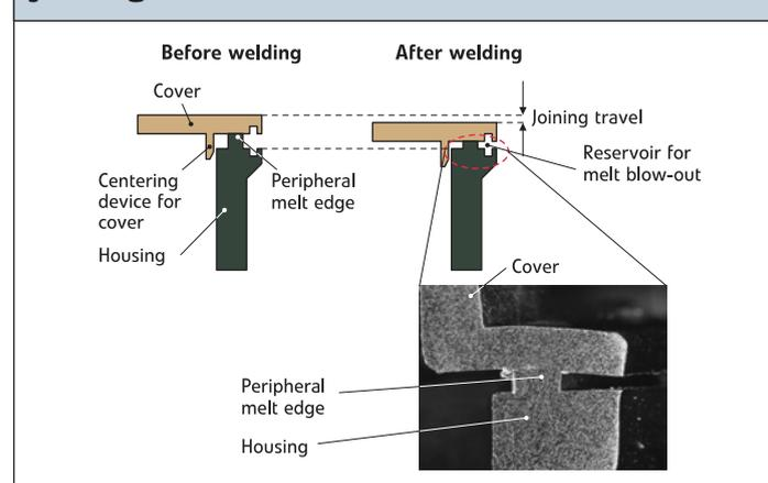
Fig. 1. Measurements of the joining distance provide information about melt flow during welding process and thus about the eventual weld [3]
